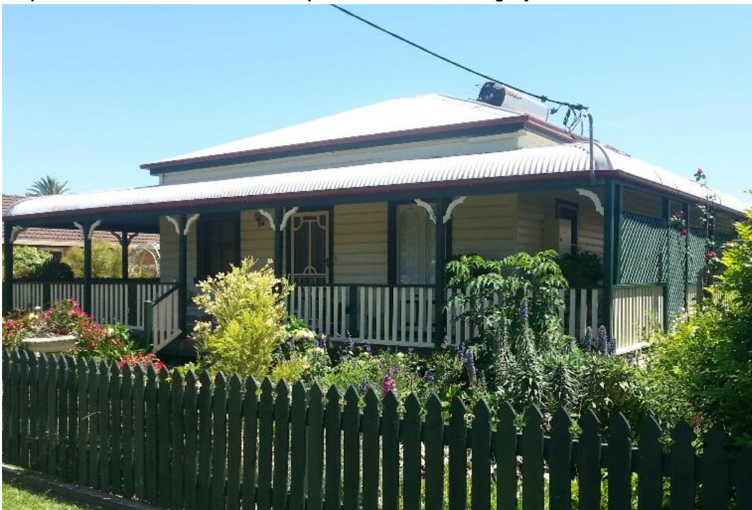
Photograph 18 - example of a dwelling circa 1900, piers, light weight building materials and wrap around verandas have been incorporated into this building style
