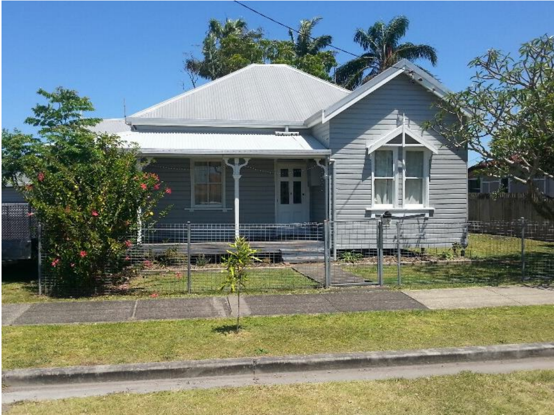
Photograph 17 – Typical workers dwelling of late 1800's early 1900's period. Use of piers and light weight materials are examples of resilient design features
