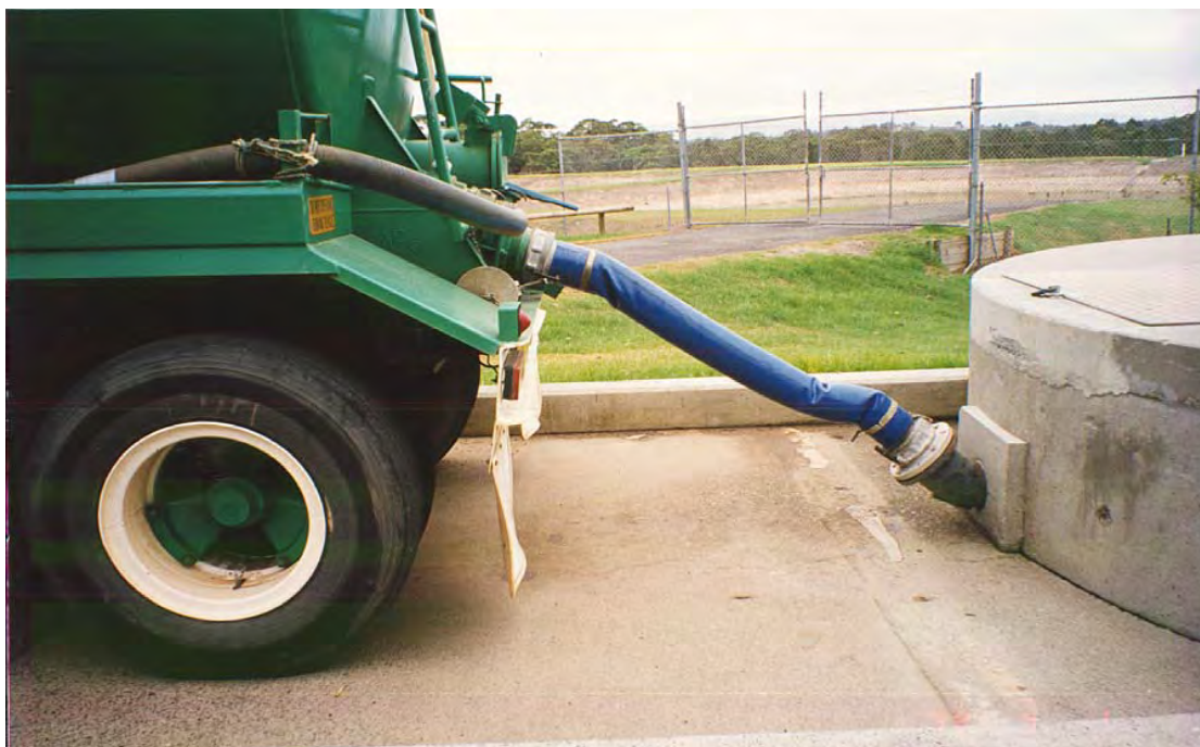
Figure 7: Tanker unloading effluent through flexible connection and KAM-LOK coupling
